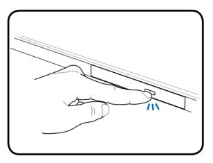
2. Gently pull on the drive's front panel and slide the tray completely out. Be careful not to touch the CD drive lens and other mechanisms. Make sure there are no obstructions that may get jammed under the drive's tray.
